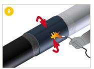
**Shrink** the heat-shrinkable sleeve around its circumference using large movements, starting at the centre.
