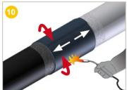
Continue heating starting from the centre and going towards the ends until shrinking is complete. Finish with horizontal movements over the whole surface of the sleeve.
