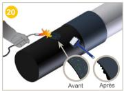
**Finalise** the bonding by warming until the coloured dots of the FOPS disappear
