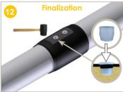
Press the female closure plugs by hand fully into the HDPE muff injection holes.
