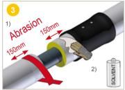
1) **Roughen** the surface (150 mm on each side) with abrasive paper or a wire brush.
