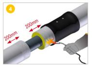
Use a blowtorch to warm the surfaces to be covered (200 mm on each end) up to at least 65 °C. Check the temperature on all surfaces with a thermometer.
