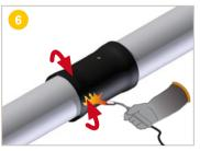
**Shrink** the ends of the heat-shrinkable muff with a blowtorch.
