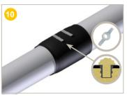
1) **Push** the 2 vent plugs fully into the 2 injection holes.
