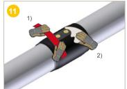
1) **Roughen** the surfaces to be covered (hole Ø + 50 mm on each side) with abrasive paper or a wire brush.
