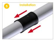
Slide the heat-shrinkable muff at the stripped area so that it covers the pipe casing by 5 to 10 cm on each end.
