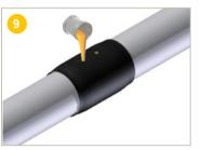
**Pour** the mixture into one of the 26 mm diameter HDPE muff injection holes. Make sure to pour in all of the mixture, using the spatula supplied.
