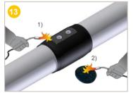
1) Use a blowtorch to warm the surfaces to be covered (hole  $\emptyset$  + 50 mm on each side) up to at least 65 °C.
