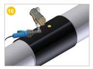
Use a punch to remove the weld-on closure plug previously heated in the welding machine.
