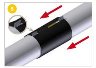
**Slide** the muff at the stripped area so that it covers the pipe casing by 5 to 10 cm on each end.
