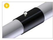
Drill a 1st hole in the muff with an electric drill, taking care not to drill the weld of the longitudinal cut.
