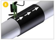
**Weld** the longitudinal cut of the muff using a PE extrusion gun.
