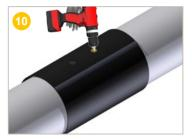
After conducting the airtightness test and demonstrating that the junction is airtight . drill the 2nd hole in the muff
