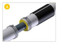
**Position** the fusion grids using the marking made previously and staple them into position.
