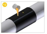
Pour the mixture into one of the 26 mm diameter HDPE muff injection holes. Make sure all of the mixture is removed, using the spatula supplied.
