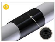
The system is correctly installed when 2 homogeneous weld beads are visible around the entire circumference of the weld-on plugs.
