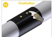
Clean the surface to remove any polyethylene or sand particles with a dry cloth (or blow off with the flame).
