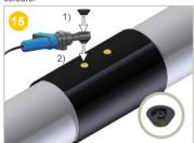
1) Use a suitable tool to place the 1st weld-on closure plug in the base of the welding machine to heat it up.
