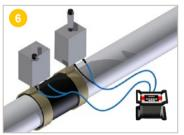
Fit the Kevlar tightening system and mount the welding tools on the muff.
