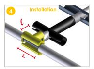
**Measure** the bare surface to be insulated then cut the half-shells to the required length (L and I).
