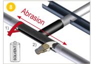
1) **Roughen** the surfaces (muff + casing 50 mm on each side) with abrasive paper (grain 40-60) or a wire brush.
