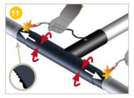
Continue heating starting from the centre and going towards the ends until shrinking is complete. Finish with horizontal movements over the whole surface of the sleeve.
