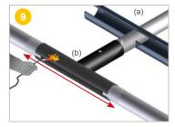
Use a blowtorch to warm the surfaces to be covered (50 mm casing + muff width) up to at least 65  $^\circ$ C.
