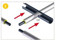
**Slide** the large heat-shrinkable sleeve (a) onto the branch pipe.
