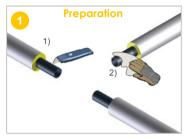
1) **Scrape** the PUR foam off the front (all signs of damp PUR foam must be removed from the 3 ends).
