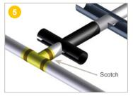
Hold the half-shells in position using sellotape.
