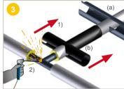
1) **Slide** the T-shaped non-drilled HDPE muff (b) onto the branch pipe.
