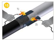
Leave 1 to 2 cm clearance to ensure correct shrinkage.
