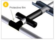
**Wrap** with the protective film supplied to avoid damaging the half-shells.
