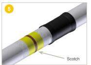
Hold the half-shells in position using sellotape.
