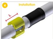
Measure the bare surface to be insulated then cut the half-shells to the required length (L). Position the 2 half-shells, checking that they fill the space to be insulated perfectly.
