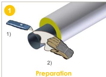
2) **Scrape** the PUR foam off the front (all signs of damp PUR foam must be removed from the ends).
