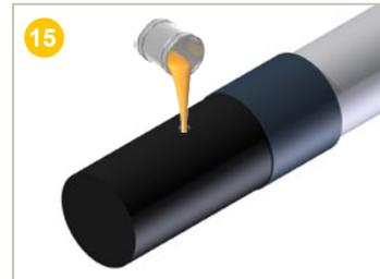
**Pour** the mixture into one of the 26 mm diameter HDPE end of line muff injection holes. Make sure all of the mixture is removed, using the spatula supplied.
