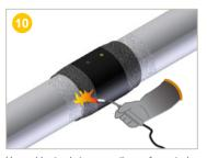
Use a blowtorch to warm the surfaces to be covered (muff + casing 50 mm on each end) up to at least 65  $^{\circ}\text{C}.$
