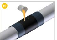
**Pour** the mixture into one of the 26 mm diameter HDPE muff injection holes. Make sure to pour in all of the mixture, using
