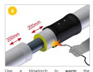
Use a blowtorch to warm the surfaces to be covered (200 mm on each end) up to at least 65 °C. Check the temperature on all surfaces with a thermometer.
