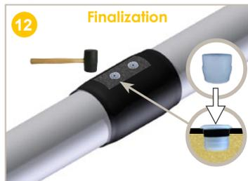
1) **Press** the female closure plugs by hand fully into the HDPE muff injection holes.
