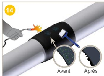
1) Finalise the bonding by **warming** until the coloured dots of the FOPS disappear.
