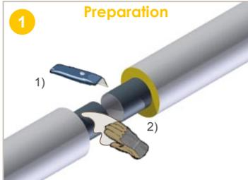
1) **Scrape** the PUR foam off the front (all signs of damp PUR foam must be removed from the ends).
