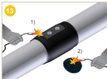
1) Use a blowtorch to **warm** the surfaces to be covered (hole  $\varnothing$  + 50 mm on each side) up to at least 65 °C.
