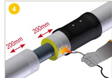
Use a blowtorch to **warm** the surfaces to be covered (200 mm on each end) up to at least 65 °C. **Check** the temperature on all surfaces with a thermometer.
