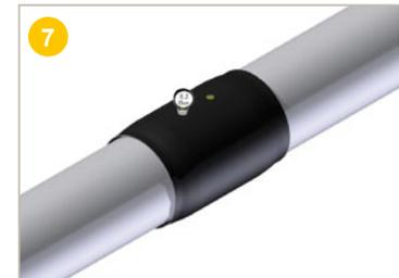
Allow to cool before injection. After shrinking and return to ambient temperature, check that the muff and the casing are firmly bonded together.
