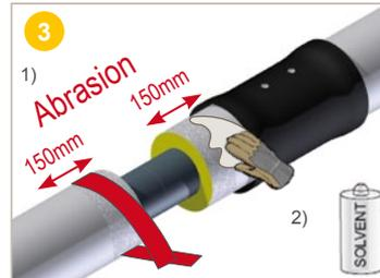
1) **Roughen** the surface (150 mm on each side) with abrasive paper or a wire brush.
