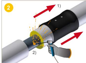
1) **Slide** the heat-shrinkable muff onto one of the pipes, **pushing it along a sufficient distance**.
