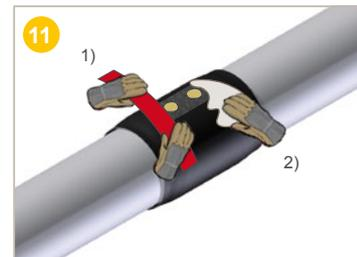
1) **Roughen** the surfaces to be covered (hole  $\varnothing$  + 50 mm on each side) with abrasive paper or a wire brush.
