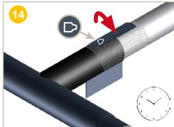
Fit the heat-shrinkable sleeve so that the overlap lies between the 10 o'clock and 2 o'clock positions. **Remember to remove its protective film.**
