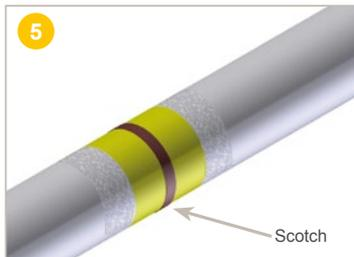
**Hold** the half-shells in position using sellotape.
