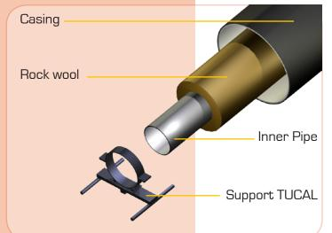
Double sleeve system for pre-insulated networks
