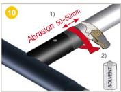
1) **Roughen** the surfaces (50 mm muff + 50 mm casing) with abrasive paper (grain 40-60) or a wire brush.
