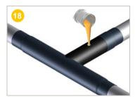
**Pour** the mixture into one of the 26 mm diameter HDPE end of line muff injection holes.
