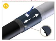
Use the application roller to smooth and evacuate the air bubbles. Use the same procedure on the closure.
