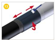
**Press** both ends of the heat-shrinkable sleeve firmly.
