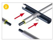
**Slide** the large heat-shrinkable sleeve (a) onto the branch pipe.
