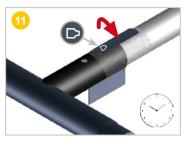
Fit the heat-shrinkable sleeve so that the overlap lies between the 10 o'clock and 2 o'clock positions.
