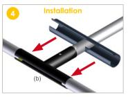
Slide the T-shaped HDPE muff (b) and fit it on the tapping.
