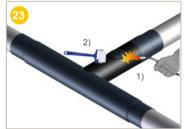
Finalise the bonding by warming until the coloured dots of the FOPS disappear
