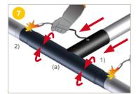
1) **Slide** the large heat-shrinkable sleeve (a) around the T-shaped HDPE muff (b).
