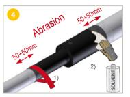
1) **Roughen** the surfaces (muff + casing 50 mm on each side) with abrasive paper (grain 40-60) or a wire brush.
