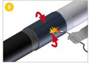
**Shrink** the heat-shrinkable sleeve around its circumference using large movements, starting at the centre.
