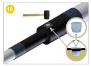
1) **Press** the female closure plug by hand fully into the HDPE muff injection hole.
