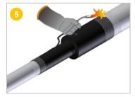
Use a blowtorch to **warm** the surfaces to be covered (muff + casing 50 mm on each side) up to at least 65 °C.
