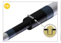
1) **Push** the vent plug fully into the injection hole.
