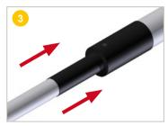
Slide the HDPE reduced muff at the stripped area so that it covers the pipe casing by 10 cm on each end.
