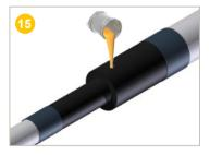
**Pour** the mixture into one of the 26 mm diameter HDPE end of line muff injection holes.
