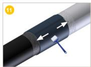
While the sleeve surface is still hot and malleable, use the application roller to **smooth and evacuate** the air bubbles. Use the same procedure on the closure.
