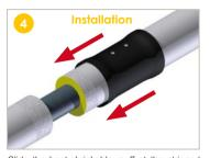
Slide the heat-shrinkable muff at the stripped area so that it covers the pipe casing by 5 to 10 cm on each end.
