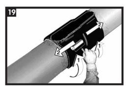
When the muff is still hot and soft, use an application roller to smooth the muff and evacuate the air entrapments.
