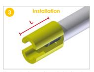
Measure the bare surface to be insulated then cut the half-shells to the required length (L). Position the 2 half-shells, checking that they fill the space to be insulated perfectly.
