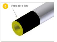
Wrap with the protective film supplied to avoid damaging the half-shells.
