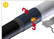
Shrink the heat-shrinkable sleeve around its circumference using large movements, starting at the centre. Depending on the diameter, use a single blowtorch for diameters <= 450 mm and 2 blowtorches for diameters > 450 mm.
