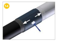
While the sleeve surface is still hot and malleable, use the application roller to **smooth** and **evacuate** the air bubbles.
