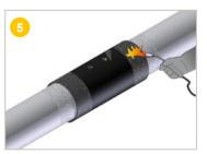
Use a blowtorch to warm the surfaces to be covered (muff + casing 50 mm on each end) up to at least 65 °C.
