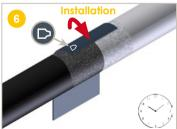
Fit the heat-shrinkable sleeve on the joint so that the overlap lies between the 10 o'clock and 2 o'clock positions
