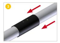
Slide the HDPE muff at the stripped area so that it covers the pipe casing by 10 cm on each end.
